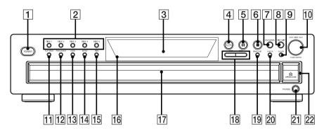
CHECK 20 (11, 12) CLEAR 9 (11, 12) DISC 1–5 2 (7, 8, 11) Disc compartment 17 (7) DISC SKIP 8 (7, 10, 12) Display 3 (9) EX-CHANGE 7 (10, 13) FADER 13 (12) PEAK SEARCH 12 (13)
